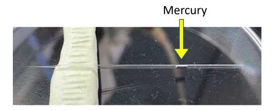
Glass pipette filled with mercury
